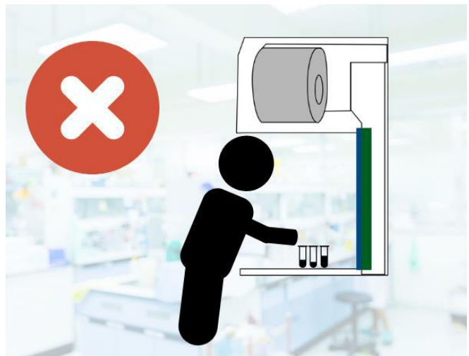
Figure 2: Incorrect position when working in the Laminar Flow Cabinet
