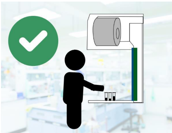
Figure 1: Correct position when working in the Laminar Flow Cabinet
